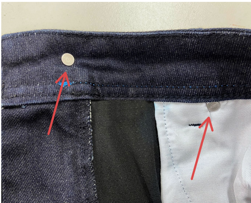
Figure 2.9: Uncovered metal fly button (left) and rivet (right) allow heat transfer to the skin in protective denim pants.
